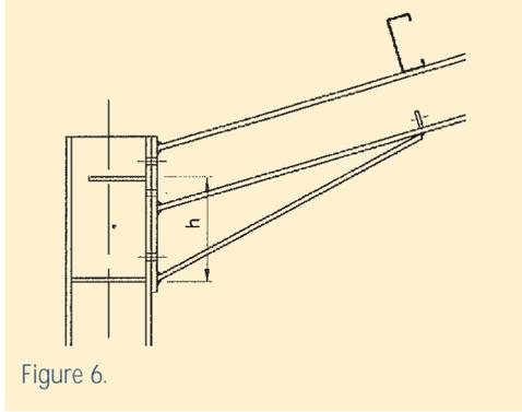
bracings or for portal rafters to columns. To make connection design readily understandable for all parties, the moments are assumed to be carried by the flanges and are connected through the end plates to the receiving (column say) member. The shear would be carried by the web (bolts).
