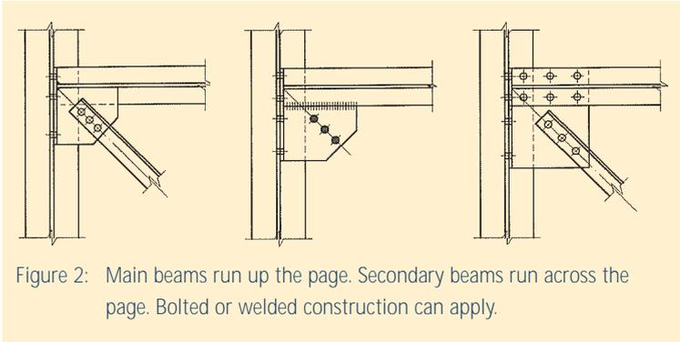
Figure 2: Main beams run up the page. Secondary beams run across the page. Bolted or welded construction can apply.
